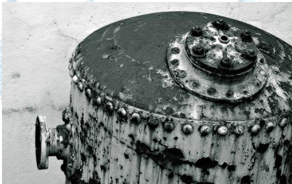
Riveted pressure vessel (left) and first welded Pressure Vessel (right).
